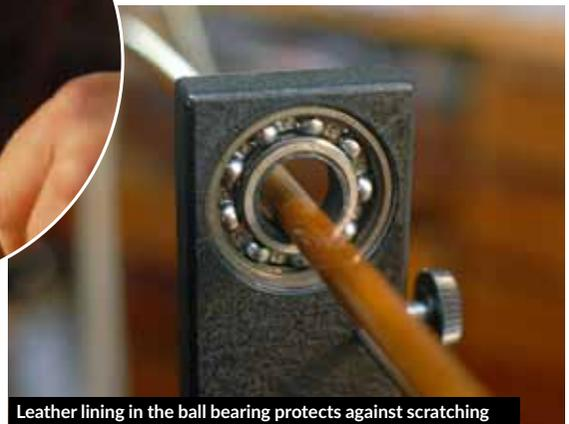
Leather lining in the ball bearing protects against scratching
