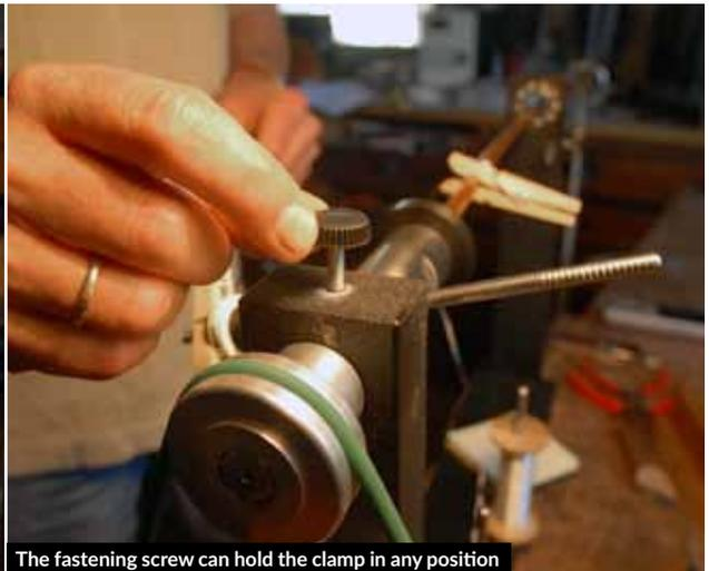
The fastening screw can hold the clamp in any position
