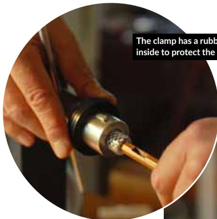
The clamp has a rubber sleeve inside to protect the bow
